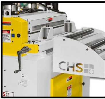
Single roll edge guides with individual or simultaneous roll adjustments
