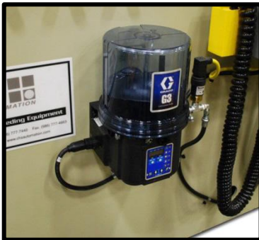
Automatic lubrication unit
