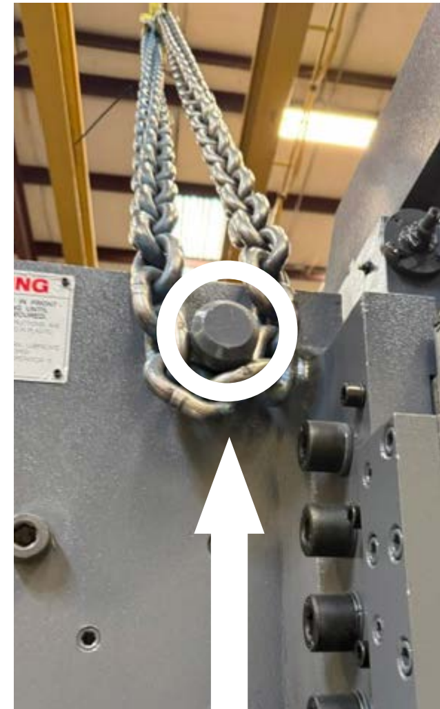
Lifting lugs are located on right side of machine
