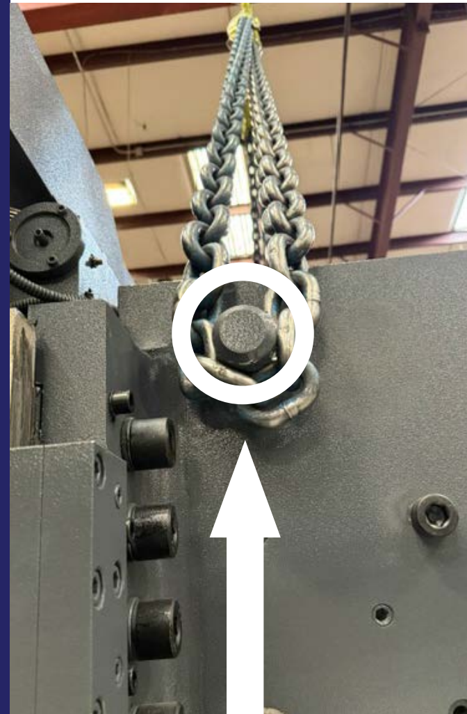
Lifting lugs are located on left side of machine
