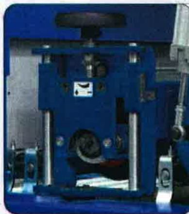
Longitudinal brush unit Ø 180 mm with height adjustment and mechanical thickness read-out. Lateral brush oscillation system. Our brushes are available in various materials: steel, stainless steel, scotch brite™, and many other.
