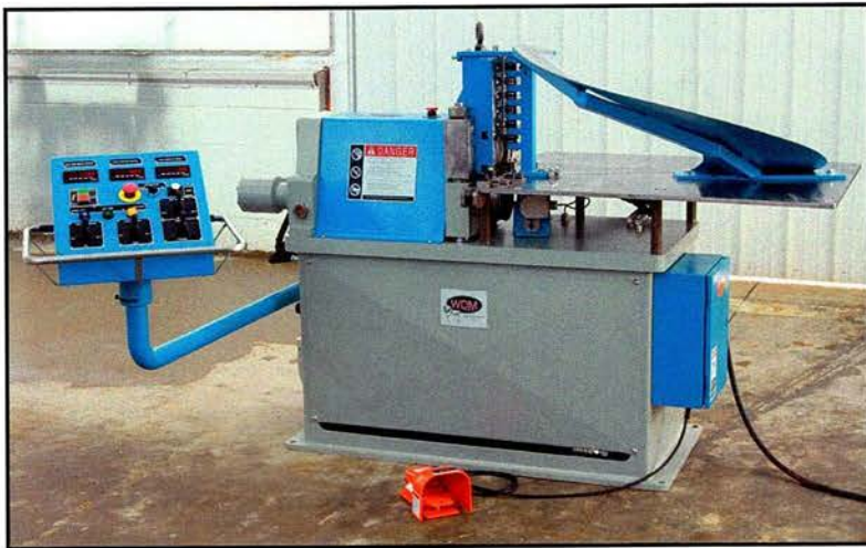
FA-7 flange forming machine making firepit ring inserts
