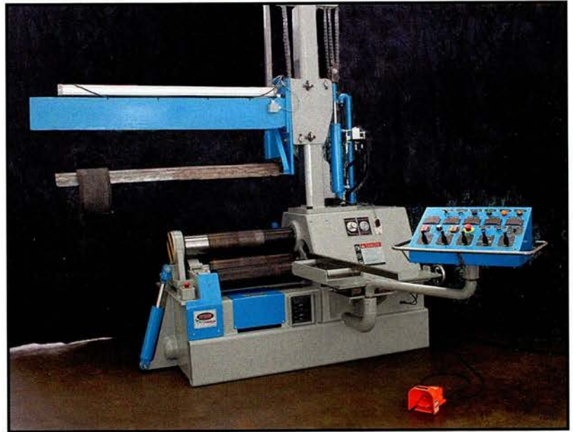
403-8(6)-2 with infeed table and overhead/ejector rolling manhole cover risers
