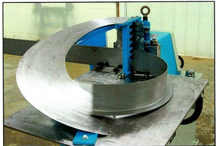
FA-7 flange forming machine making firepit ring inserts
