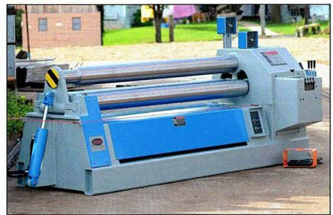
101-6-6 Plate Roll w/Rotation Foot Switch and Manual Hydraulic Valves
