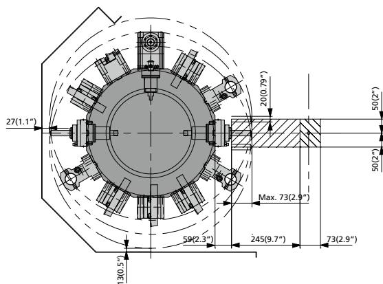
Angular Milling Tool (Y-Axis)
