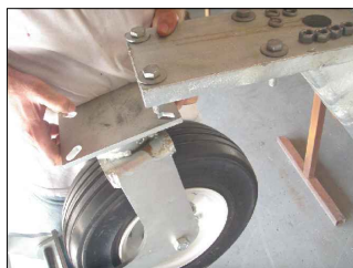
ALIGN SWIVEL WHEEL AND BOLT TO GOOSENECK WITH \frac{1}{2} X2 \frac{1}{2} BOLTS
