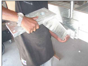
ALIGN HOLES IN GOOSENECK, CHARIOT BRACKET, AND BASE
