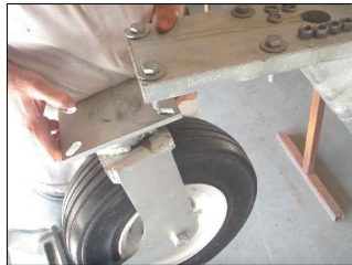
ALIGN SWIVEL WHEEL AND BOLT TO GOOSENECK WITH \frac{1}{2} X2 \frac{1}{4} BOLTS
