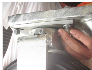
TIGHTEN ALL (4) CONNECTIONS WITH SOCKET AND WRENCH
