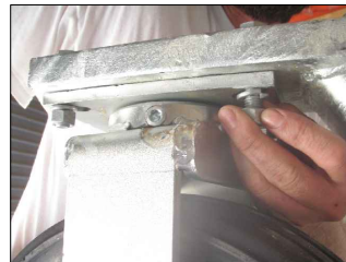
TIGHTEN ALL (4) CONNECTIONS WITH SOCKET AND WRENCH
