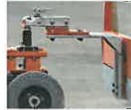
ALIGN DOLLY MOUNT PLATE AND BOLT TO TOP OF GOOSENECK WITH \frac{1}{2} "X2 \frac{1}{4} " BOLTS AS SHOWN
