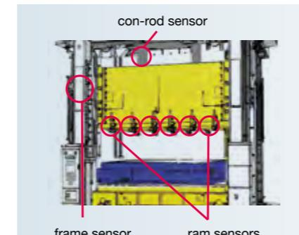
The sensor type and its position are determined by the respective monitoring task.
