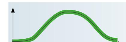
The process signals are taught-in during good part production and limits (envelope curves, etc.) of faultless production are calculated automatically.
