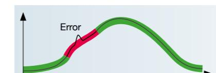
If one of the monitoring limits (e.g. envelope curve) is exceeded, the part is sorted out or the machine is stopped.
