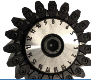
Inserted Skiving Mills (Module 4 and larger) IT8/IT9 Cutting speed 160-260 m/min (dry machining)
