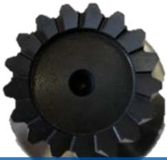
Coated Powder Metal Steels (PM) Skiving Mills < IT8 Cutting speed 100-160 m/min
