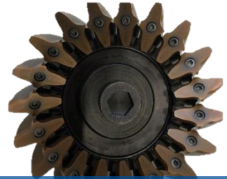
Inserted Skiving Mills (Module 4 and larger) IT8/IT9 Cutting speed 160-260 m/min (dry machining)
