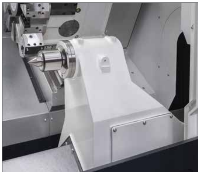
NC SERVO-DRIVEN TAILSTOCK
