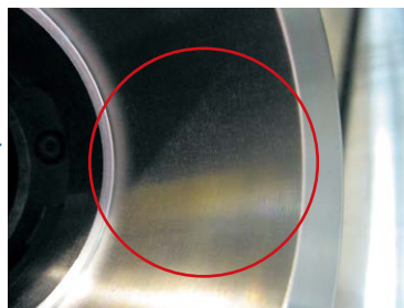
Smooth surface, clean finished threads
