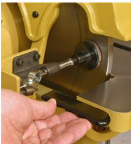
This hand-operated disc brake lets the operator stop the heavy platen in seconds and do it safely.
