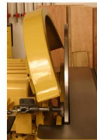
The thick, steel platen is precision machined and balanced to virtually eliminate vibrations. Notice how the disc guard tilts back out of the way to ease changing abrasive discs.
