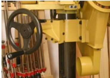
The table is raised and lowered using this rack and pinion system, operated by the large handwheel. Also, you can see the 4"-diameter dust port.
