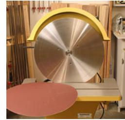
The spacious cast iron table tilts 30-degrees up and 45-degrees down for easy bevel sanding of virtually any angle. The table also can be raised and lowered for maximum versatility and for changing abrasive discs.
