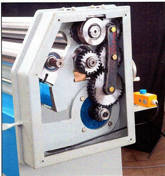
Heavy duty all-gear drive for roll rotation 2-roll drive.
