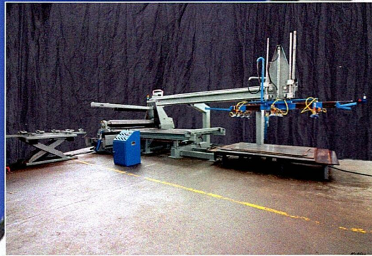
403-13-8 rolling cell to form propane tanks
