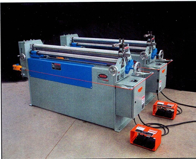
Completed 310-2.6-48 (20 gauge X 4') to make ducts for the HVAC industry
