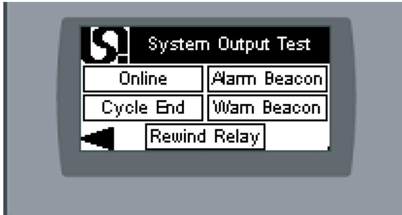
All buttons on this screen are momentary; in other words the output will only be on while you hold the button). While this screen is displayed, all automatic control of the PLC outputs is disabled
