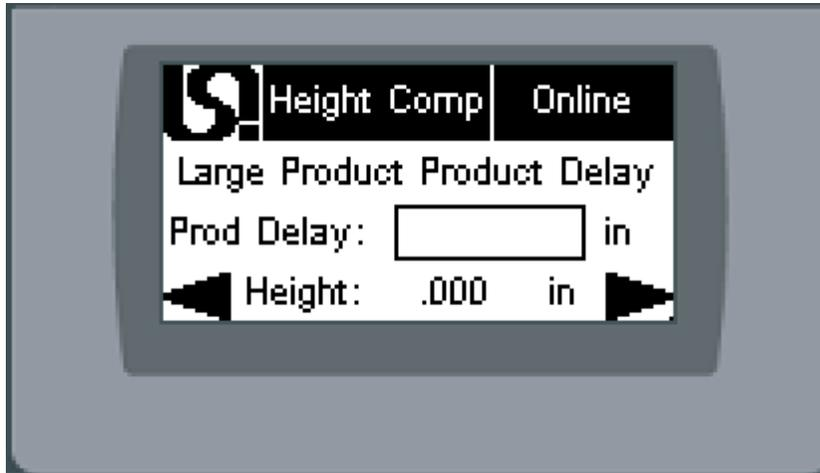
**NOTE: For Height Comp to work properly, Product Delay must be set on both Height Comp Screens (Small Product Product Delay and Large Product Product Delay Screens). Height Comp disabled in this screen for set up purposes.**
