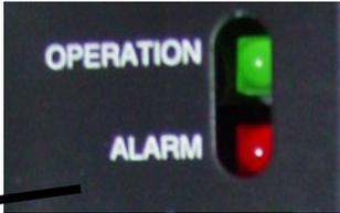
The front panel of the drive includes 2 LED indicator lights. The Operation indicator illuminates to indicate that 120 VAC power is being supplied to the unit. The Alarm indicator blinks when a protective function is triggered
