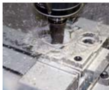
Large hole drilling using high-torque specs Hole diameter : \phi 40 mm Material: Carbon steel
