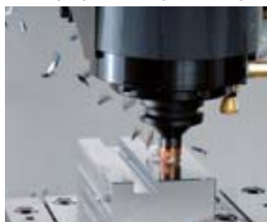
Grooving using standard specs Cutting amount : 150cc/min Material: Carbon steel (for \phi 16 end mill)
