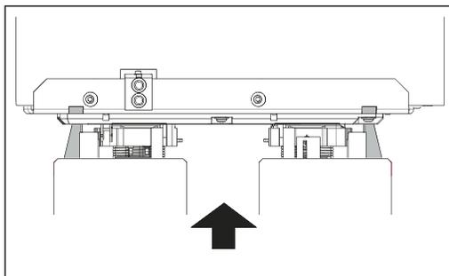
When the print heads make contact with the cap unit, turn the cap-unit tool one or two turns more.
