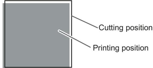
Printing position and Cutting position are misaligned.
