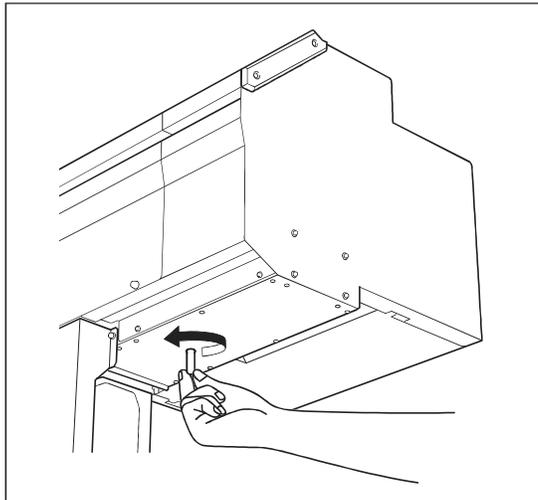
Insert the cap-unit tool into the hole at the bottom of the machine and turn gently. The cap unit rises.
