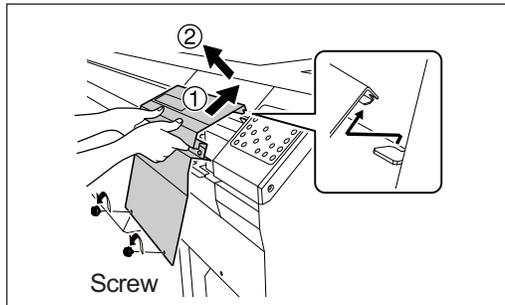
Remove the screws, lift the cover R in the direction of ①, and then pull it out in the direction of ②.
