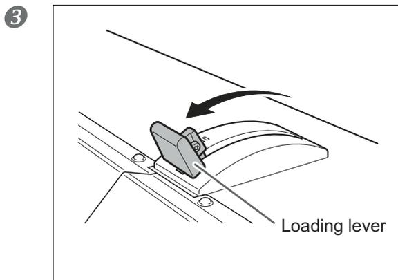
**Pull back the loading lever to secure the media in place.**
