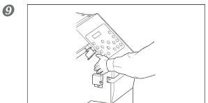
Touch the location shown in the figure to discharge any static electricity.
