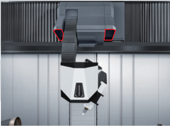
The duct, which synchronizes with the Z-axis movement of the AM head, maintains a certain distance from the machining point.
