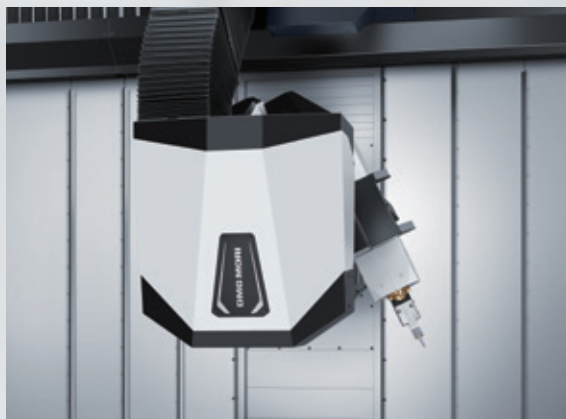
Even with an AM nozzle, the B-axis provides a wide swivel range of 240°(-30° to +210°), allowing metal deposition on the Spindle 2 side in a wide movable range.
