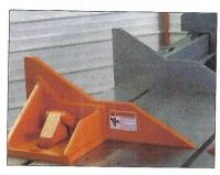
Carbide Blade Guides: Side and back carbides are flat for maximum blade support.
