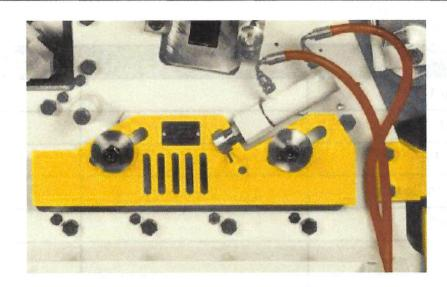
Flat Shear Hydraulic Hold Down for better holding of the material.
