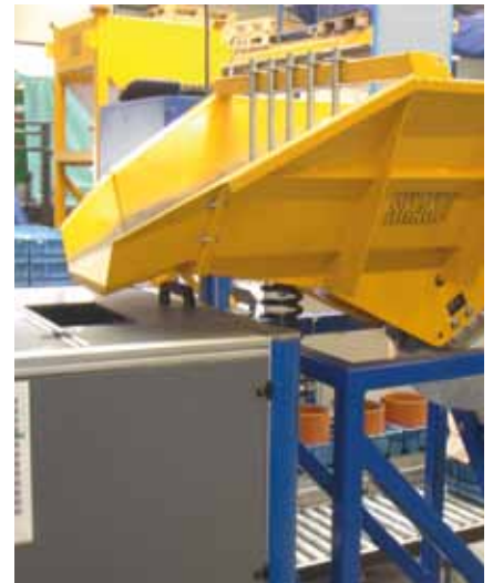
Storage feeder prior to sorting machine
