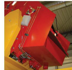
Tipping in Steps allows partial filling of e.g. the storage feeder for optimized disentangling of very difficult products.
