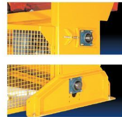
Direct Access to Chain Adjuster. Combined with the easy chain wheel repositioning, the chain adjuster indicates the exact time for chain replacement.
