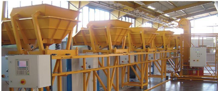
Traversable Design facilitates economic distribution of products to e.g. several in-line storage feeders.
