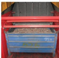
Locking Bar Arrangement manually adjustable for various container heights.
