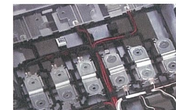
Battery pack assembly of BMW i3
