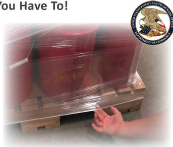
Pallet Grip rolls up a film cable and drives it down onto the pallet, locking the load. This makes sure your load does not slide off during transit.
