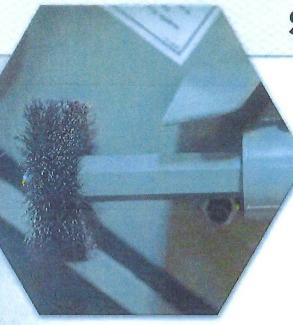
Chip Brush: Powered from the drive wheel of the saw, the brush changes speed with the blade to assure that chips are being removed from each gullet, improving cutting performance and blade life.
