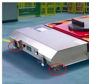
Universal Wheels: It ensures that the skate can turn smoothly while moving forward.
