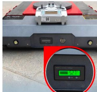
LED Display: Convenient to observe the power to remind timely charging.
