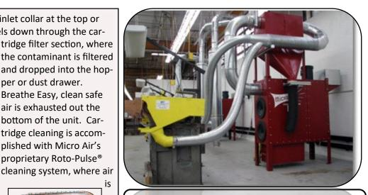
**RP2** with Spark Arrestor Ducted to **Buffing / Polishing Operations**
