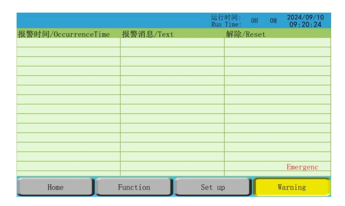
This interface shows current and history alarm records. When the equipment reports an alarm, the customer can identify the cause according to the alarming content and automatically clear the alarm or contact the manufacture.
