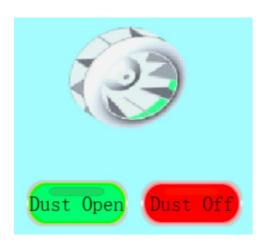
Click "Dust Open" to start the dust exhausting fan. Click "Dust Off" to stop the dust exhausting fan.
