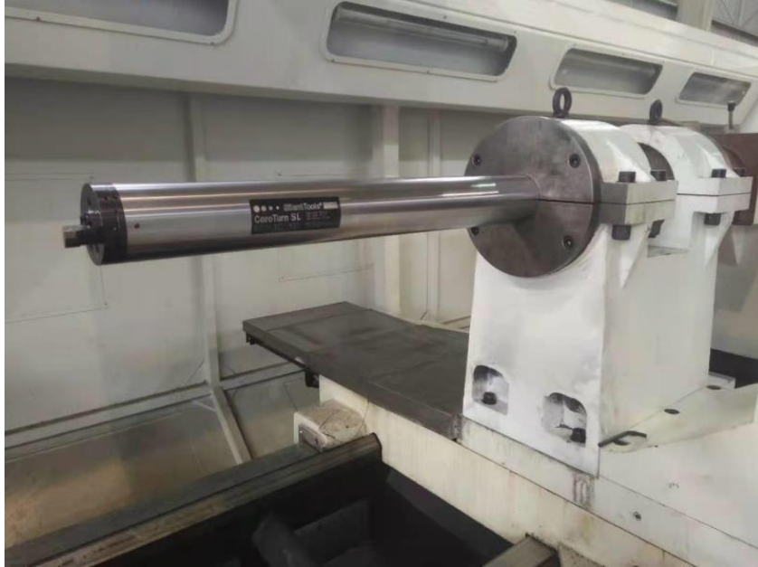
Extended Boring Bar Holder
