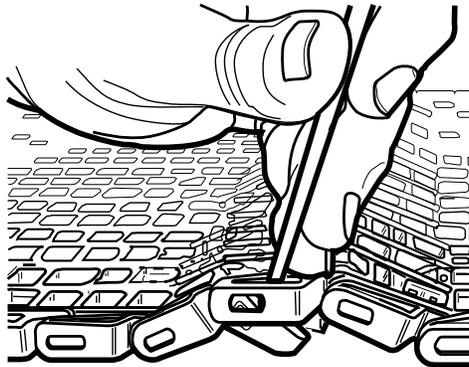
3. Continue to push down on the retainer clip to move it out of the end link.
