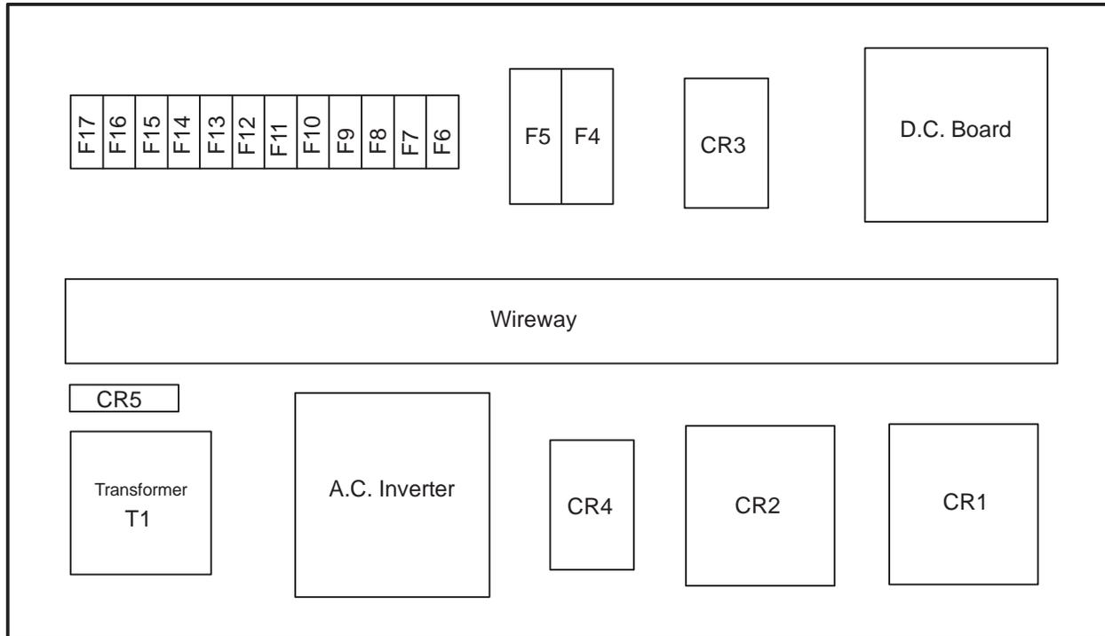
Panel layout for larger model tunnels: ETB4816, ETB4820, ETB5616, ETB5620, ETB7016 & ETB7020
