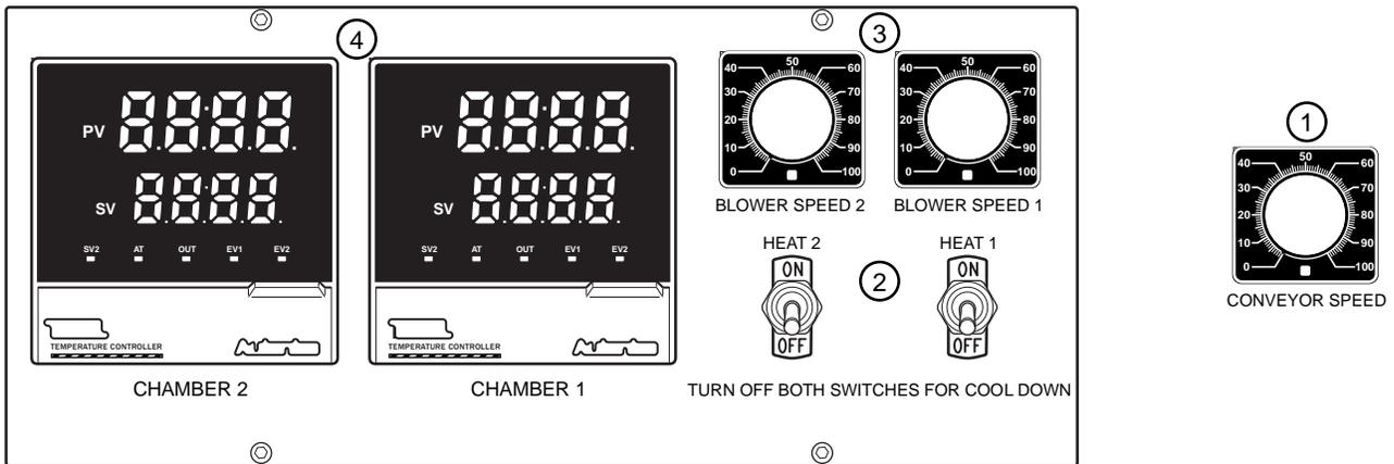
Controls for the bundling tunnel are located along the front side of the machine as shown in the figure. Controls from right to left are listed below.
