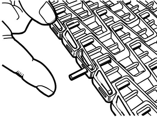
2. Insert a plastic retainer clip into place to retain the metal rod. Use a hammer, if necessary, to gently tap the retainer clip into place.
