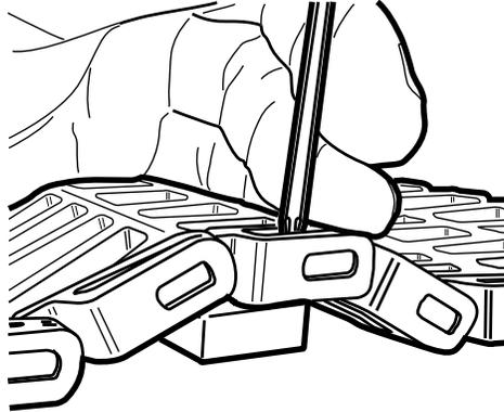
2. Use a screwdriver to push down on the retainer clip to unseat it.
