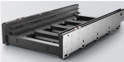
Mortise-and-tenon welding structure machine bed
