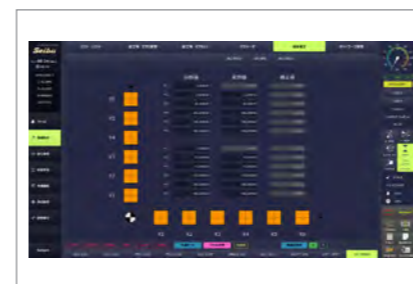
Inclination compensation software Straightness of X.Y axis can be corrected.
