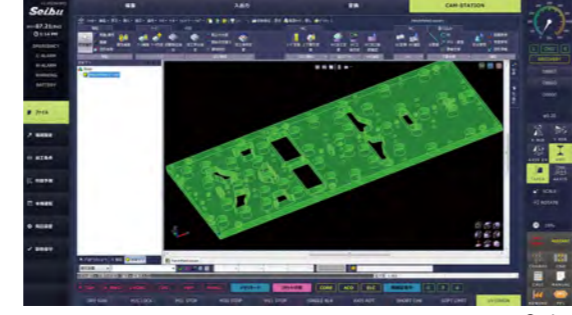
CAM-Station: NC program conversion is possible from the CAD data (2D/3D)
