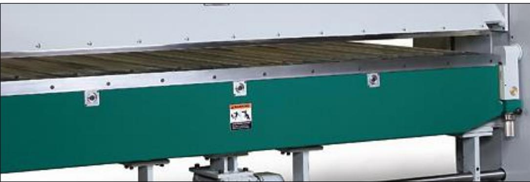
The SBS126-14 comes standard with crowning system. This crowning system gives SBS owners the most complete adjustment of any standard sheet metal folder on the
