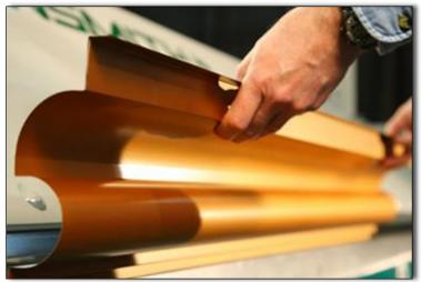
The center placement of the clamping motor also benefits the forming of radius profiles. To achieve consistent radial shapes, it is very important to have even clamping pressure. Equal clamping pressure will ensure the part is formed evenly throughout the entire profile.
