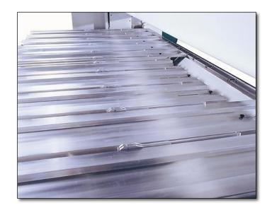
The back gauge for the SBS126 Series features a twin ball screw design. The system is fast extremely accurate and incorporates 12 solid fingers. All three drive systems of the SBS Series: Folding beam, Clamping Beam and Backgauge are controlled by frequency inverters, giving the SBS unbeatable accuracy and performance.
