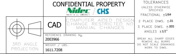
TOLERANCES UNLESS OTHERWISE SPECIFIED FRACTIONAL ±1/64 2 PLACE DIMS. ±.01 3 PLACE DIMS. ±.005 ANGLES ±1/2°
