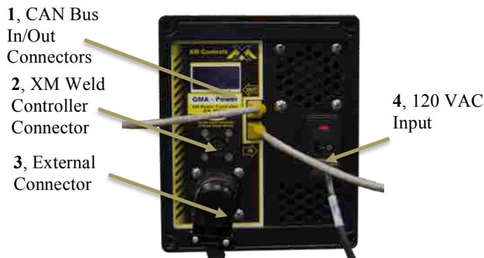
Each XM Control Module (or XM Module) is designed to control a specific component of the system (such as a welding power supply or rotation of a lathe). This makes for powerful real-time monitoring of the system as well as extremely low latency control over all automated processes. All the modules in the
