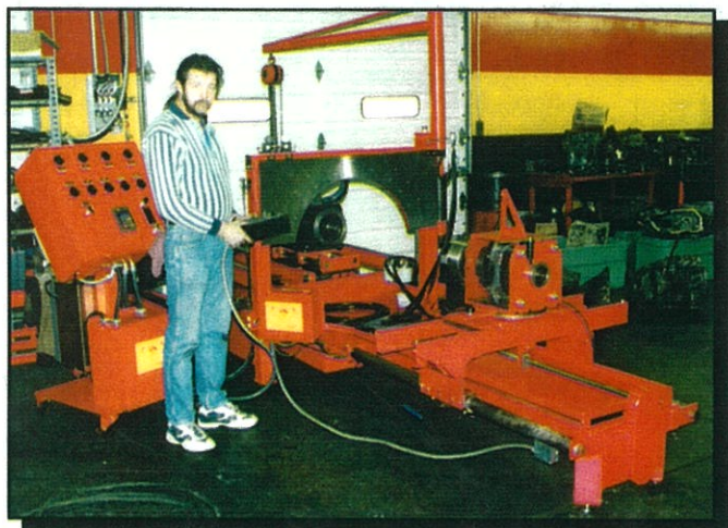
EASY ACCESS TO VALVE BODY, NO NEED TO TURN THE TRANSMISSION OVER
