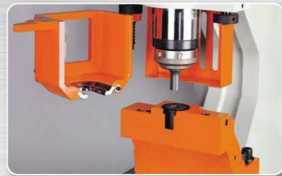
*Goose-neck die holder for punching channel flanges and webs.
