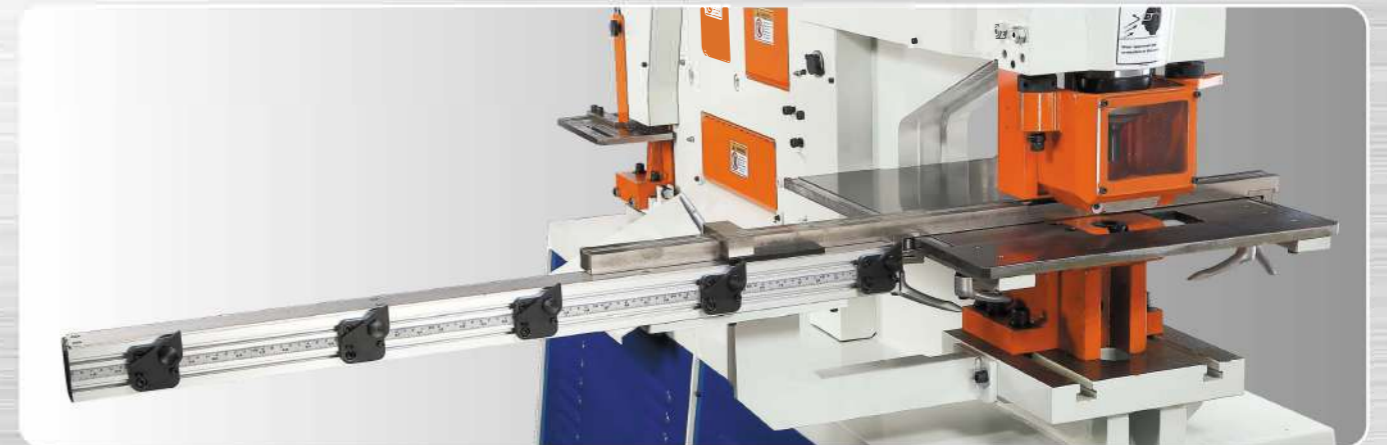
*Flip-stop gauge table. 1-3M lengths. (S/SD/KD and PM models only)
