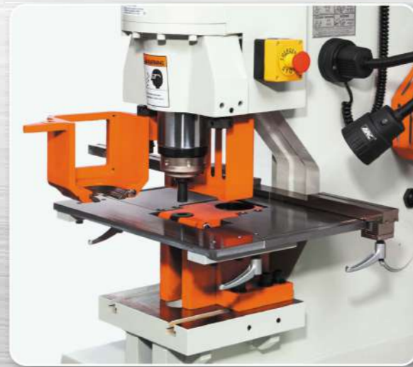
*Standard dual-opening die block for up to 2" round punch and die.
