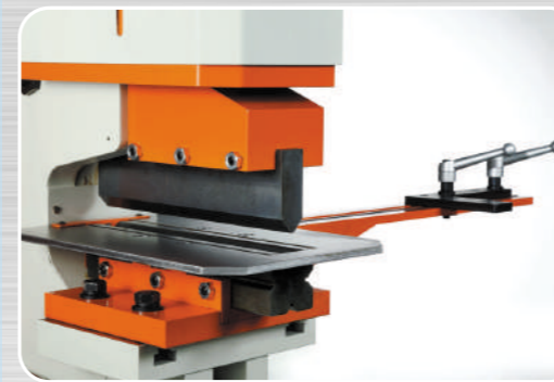
*Urethane spring stripper. Safety cover removed for showing.
