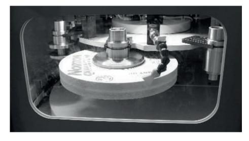
unit on a Model 1000 is a rotary dressing spindle. For even wider profiles and multiple dress rolls we can offer a variety of dual supported dresser spindles. Single point, cluster diamonds, etc. are also often added depending on customer requirements.
