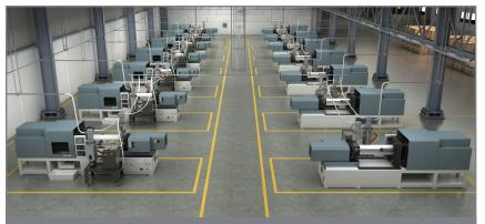
**Factory E - 7 Pump / 28 Stations** VacTrac<sup>®</sup> Plus3 - 14 AD Dryers with hoppers & receivers, 14 Machine Hoppers, and 7 Vacuum Pumps in a pumping room all conveying to 14 Injection Molding Machines.
