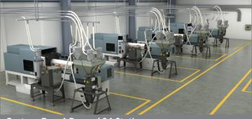
**Factory D - 4 Pump / 24 Stations** VacTrac<sup>®</sup> Plus2 - 4 AD Dryers with hoppers & receivers, 4 BD Blenders with 16 receivers, and 4 Vacuum Pumps in a pumping room all conveying to 4 Injection Molding Machines.
