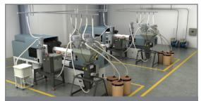
Factory B - 2 Pumps / 12 Stations VacTrac® Plus1 - 2 AD Dryers with hoppers & receivers, 2 BD Blenders with 8 receivers, and 2 Vacuum Pumps all conveying to 2 Injection Molding Machines.
