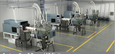
**Factory C - 3 Pump / 18 Stations** VacTrac<sup>®</sup> Plus2 - 3 AD Dryers with hoppers & receivers, 3 BD Blenders with 12 receivers, and 3 Vacuum Pumps all conveying to 3 Injection Molding Machines.
