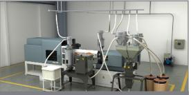
**Factory A - 1 Pump / 6 Stations** VacTrac<sup>®</sup> Plus1 - 1 AD Dryer with hopper & receiver, 1 BD Blender with 4 receivers, and 1 Vacuum Pump all conveying to an Injection Molding Machine.
