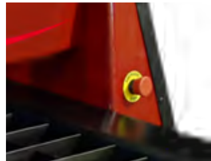
Emergency Stop Button E-stop button located on each saddle quickly and safely shuts off machine motion and cutting process, including oxy-fuel gases to the torches.
