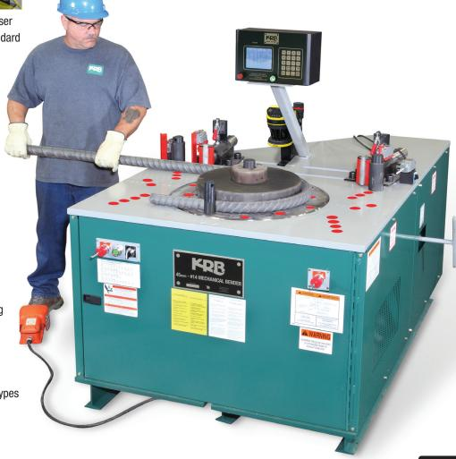
The KRB #14 Mechanical Bender is a proven workhorse for bending reinforcing bar. The rugged, heavy welded steel construction combined with simple mechanicaldrive assures continuous operation under adverse conditions. Forward or reverse bending enables all types of bending to be performed with ease.
