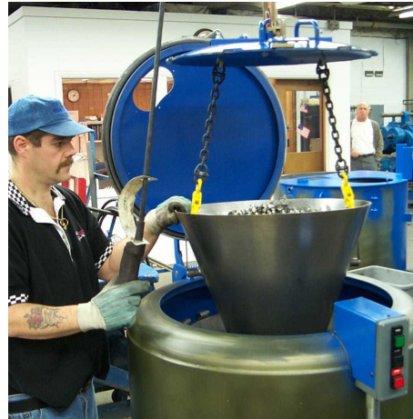
Lower pan into place
