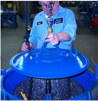
Load pan cover onto spindle
