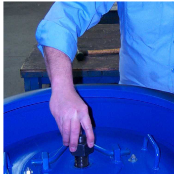
Thread spindle nut onto spindle
