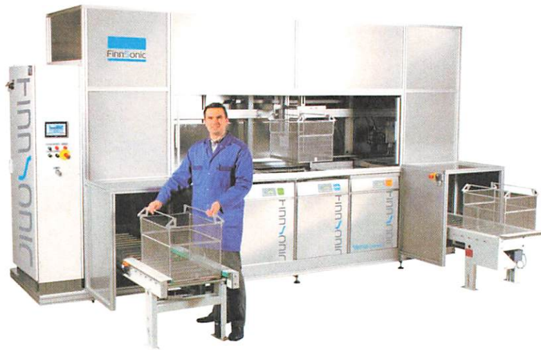
Example photo of automatic Versa Genius cleaning line with full encapsulation and TD35 basket transporter. (for illustration purposes only, not 100% identical with the quoted solution)
