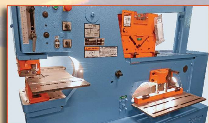
LED Work Light: Punch & Shear
