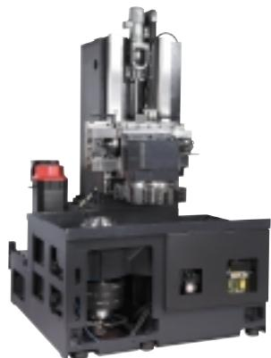
The one piece bed and box type column castings are rigid and heavily ribbed. Meehanite cast iron. These castings remain stable even under the heaviest cutting conditions. Fine grained Meehanite cast iron is used for its excellent vibration absorbing characteristics. The cross slide body is fully supported by the saddle in all positions and there is no table overhang.
