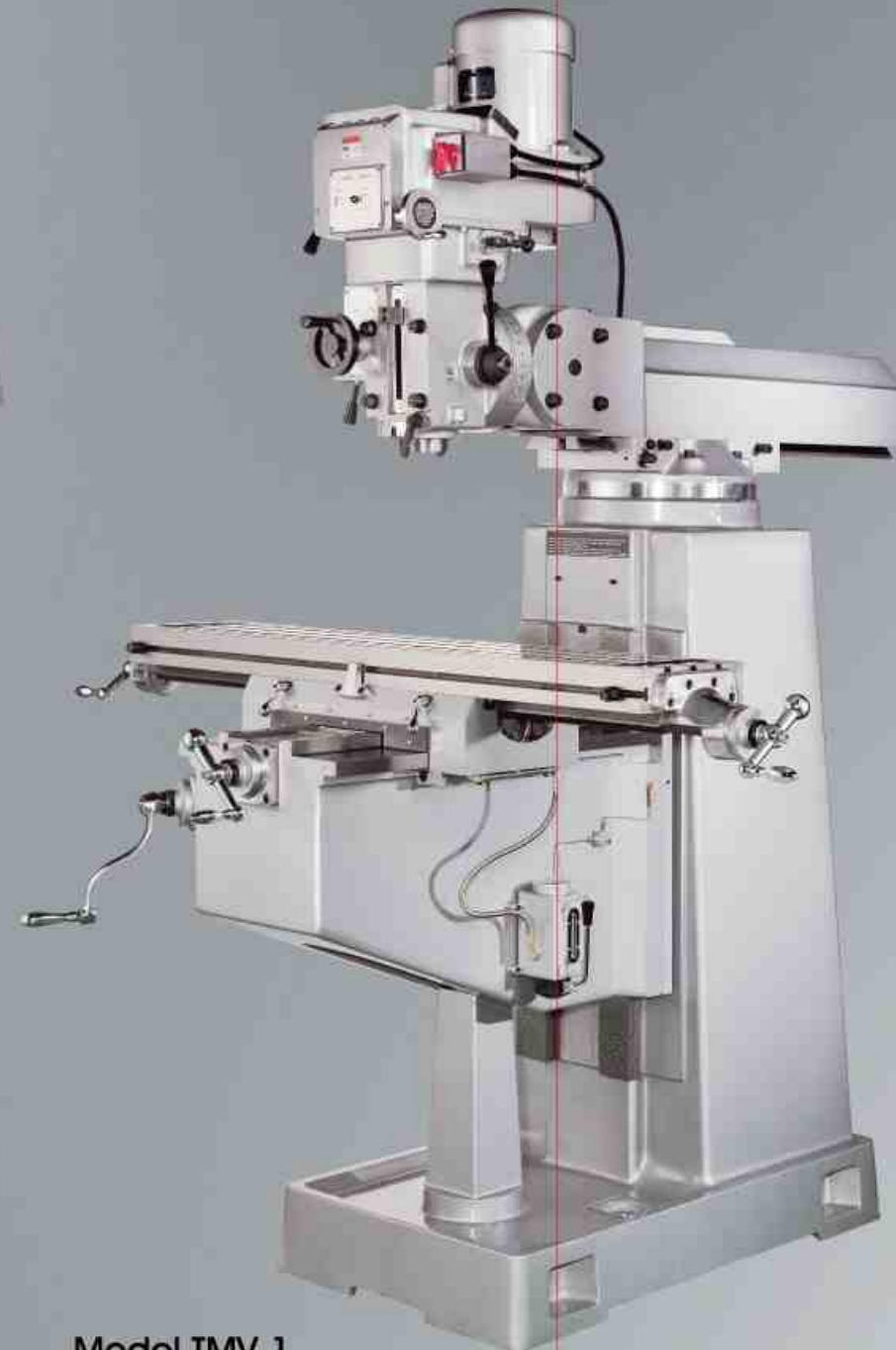
Model TMV-1 with 5 HP, #40 taper Spindle
