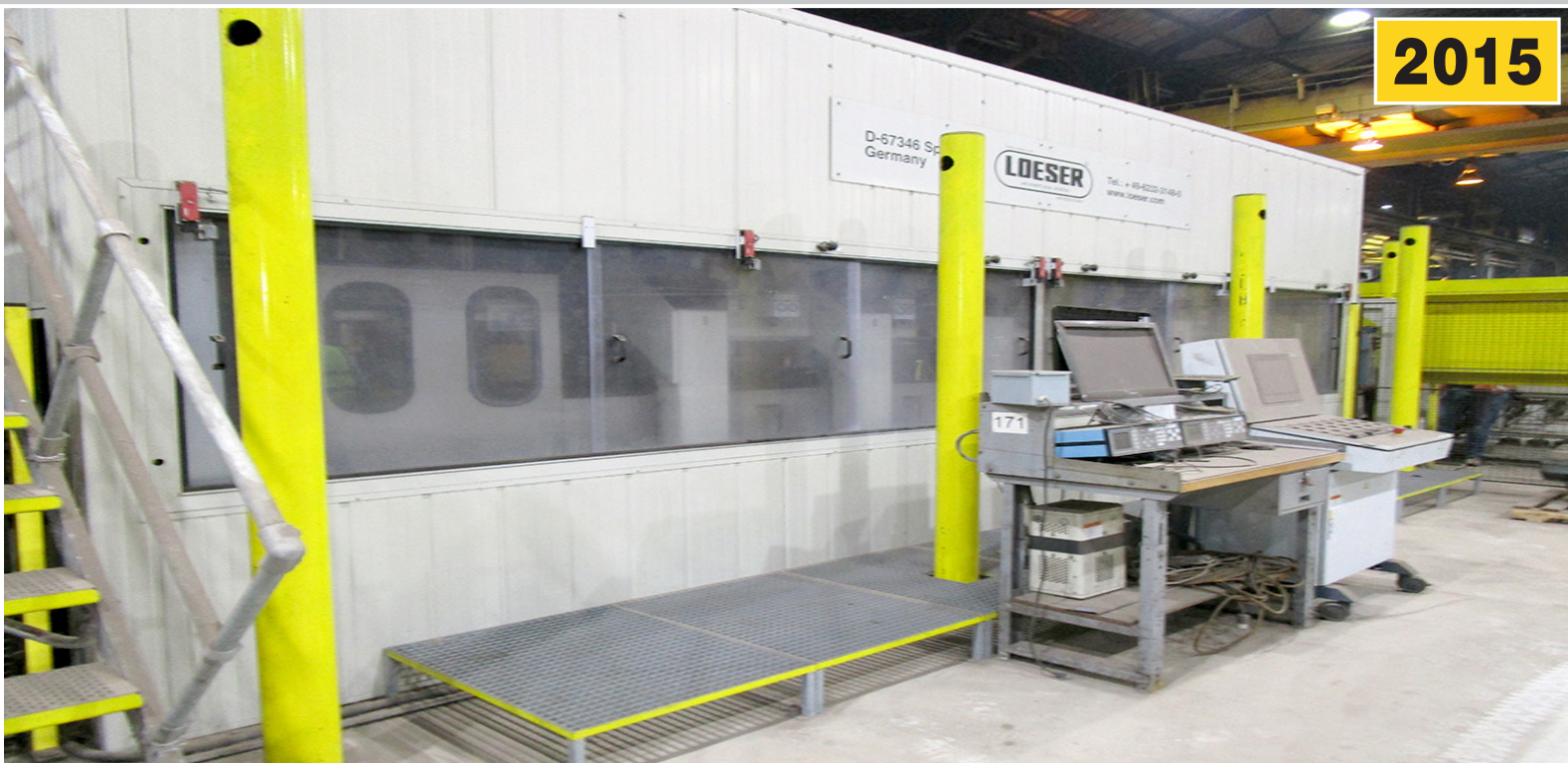
12" (300mm) LOESER Tube and Bar Grinding and Polishing Line
