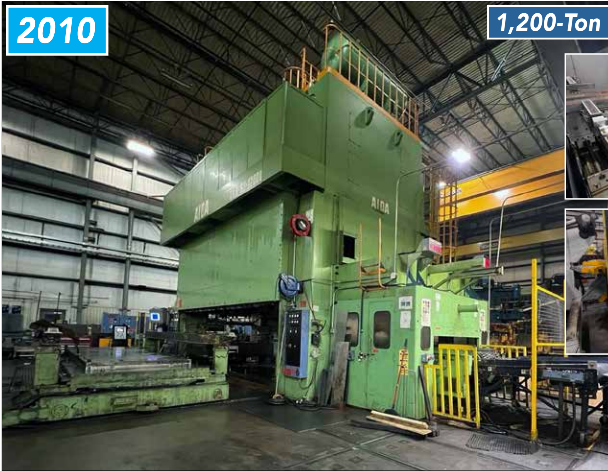
1,200-Ton Aida TMX-S2-12000 Transfer Stamping Press, with CoilTech Servo Feed Line Coil Loading Ramp, CoilTech Press Servo Straightening System and Decoiler
