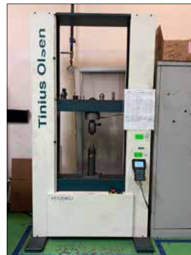
Tinius Olsen H100KU Universal Testing Machine, 100 kN Capacity, Digital Control, Floor Model
