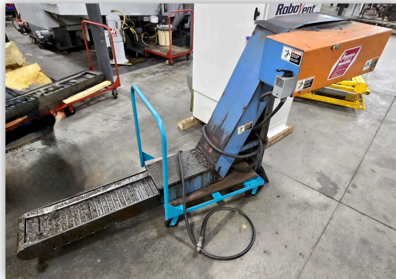
Jorgenson Chip Conveyor
