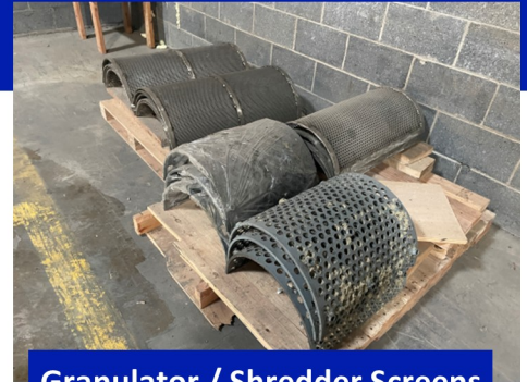
Granulator / Shredder Screens
